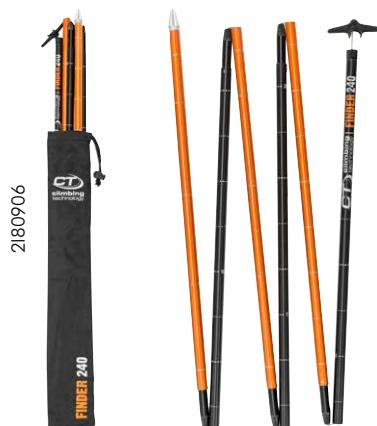
240 cm avalanche probe composed of six sections with a quick tensioning system with an internal Kevlar cord. Designed for identifying the burial point when searching for a missing person. Numerical indication included along the probe. Bag included.
