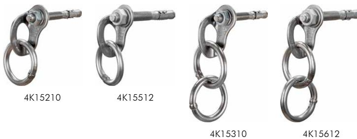
AISI 316L stainless steel anchor, consisting of a bolt with a single expansion element and a multidirectional anchor plate. Equipped with one or two rings, having inner diameter 40 mm.
