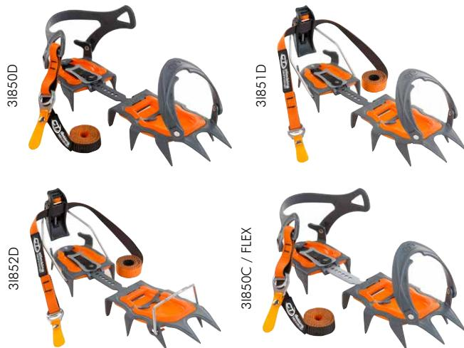
Twelve point crampons studied for classic mountaineering: Couloirs, ridge with mixed climbing and easy goulottes. Made from tempered painted steel. Shaped frontal points to enhance progression on slopes. Available also in the version with flexible adjustment bar, which enable them to be used with non-rigid boots.
