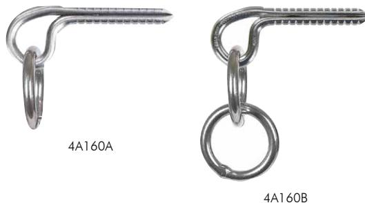
Glue-in anchor made of AISI 316L stainless steel, to be installed with chemical resin. Equipped with one or two rings, having inner diameter 40 mm. Used in pairs, it allows a belay station to be created.
